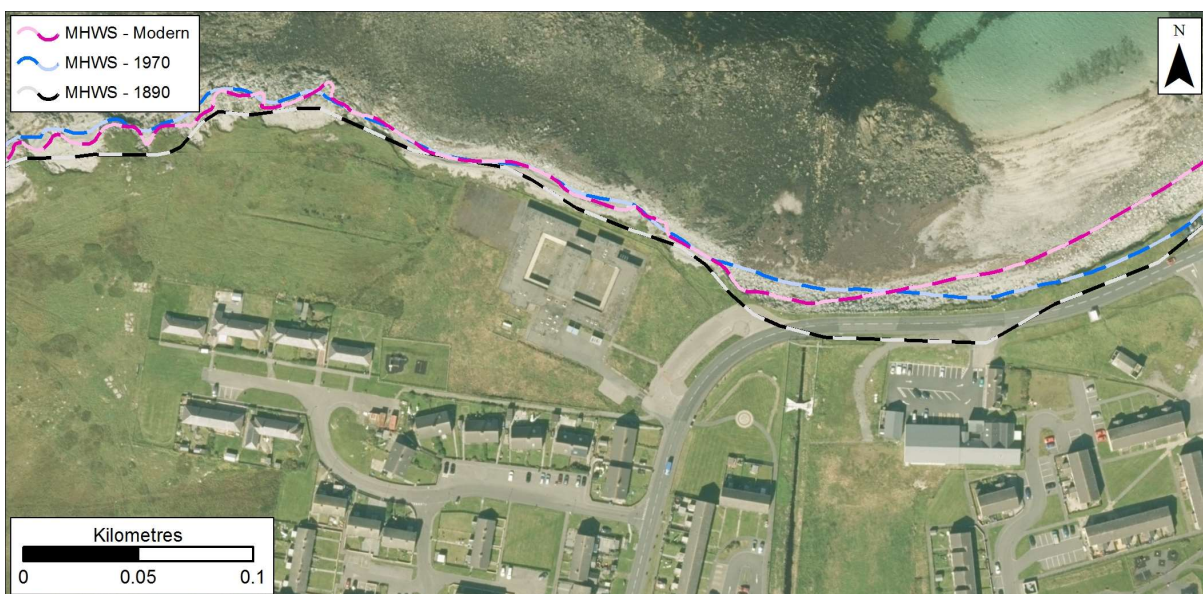
Figure 9.23: MHWS position in 1890, 1970s, and Modern datasets at Balivanich Primary School. Getmapping are our current providers of Scotland-wide digital aerial imagery© Getmapping plc.
