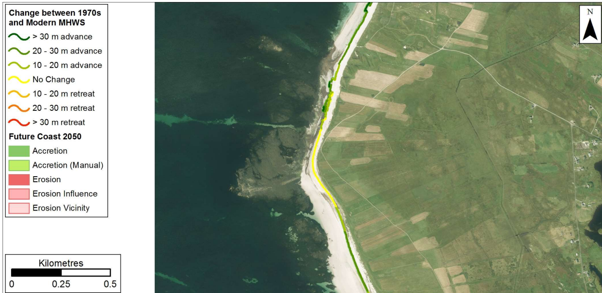
Figure 9.31: Change between the 1970 and Modern MHWS data at Kilpheder. Getmapping are our current providers of Scotland-wide digital aerial imagery© Getmapping plc.
