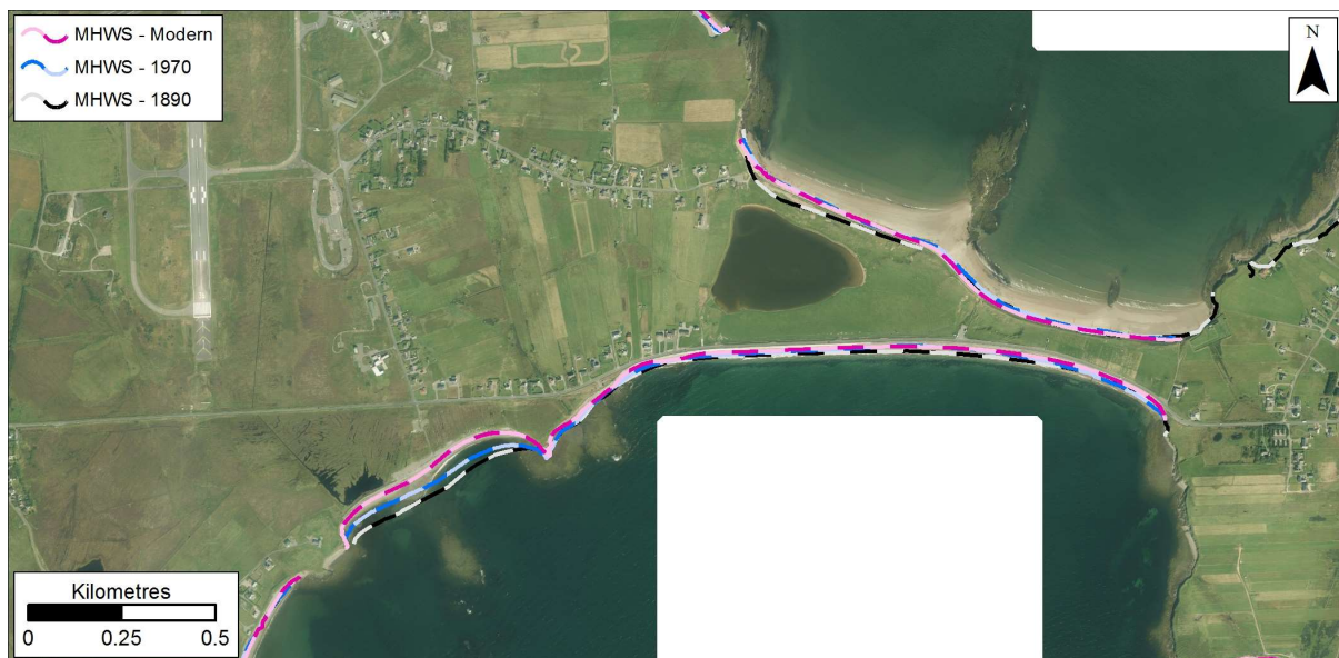
Figure 8.5: MHWS position in 1890, 1970s, and Modern datasets at the Braigh. Getmapping are our current providers of Scotland-wide digital aerial imagery © Getmapping plc.
