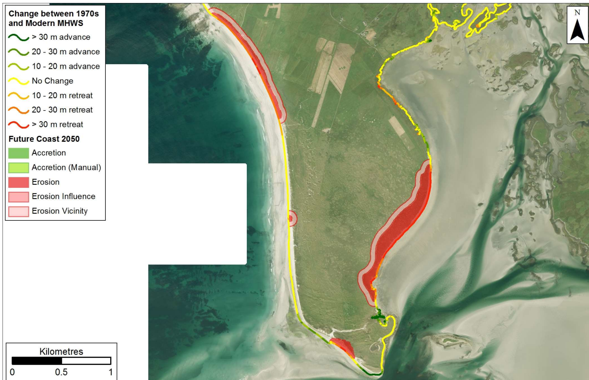
Figure 9.18: Possible future coastline position in 2050 based on rates between 1970 and Modern MHWs data at Baleshare. Getmapping are our current providers of Scotland-wide digital aerial imagery© Getmapping plc.
