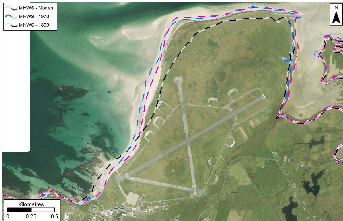
Figure 9.19: MHW position in 1890, 1970s, and Modern datasets at Benbecula Airport and Balivanich. Getmapping are our current providers of Scotland-wide digital aerial imagery© Getmapping plc.
