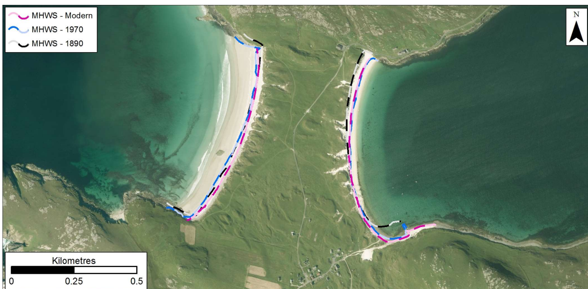
Figure 9.37: MHWS position in 1890, 1970s, and Modern datasets at Vatersay tombolo. Getmapping are our current providers of Scotland-wide digital aerial imagery © Getmapping plc.
